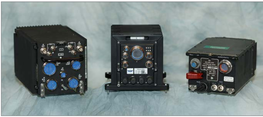
Figure 2 | TESseract mission computer from TES-SAVi with AN/ARC-231 and AN/ARC-201D radios.
